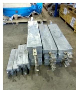
Oct 2020 - Material Sacrificial Aluminium Anode for Jembatan 2
